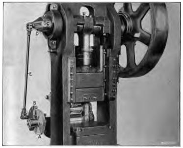
Fig. 1. Straight-sided Press Equipped with Single-roll Ratchet Feed
